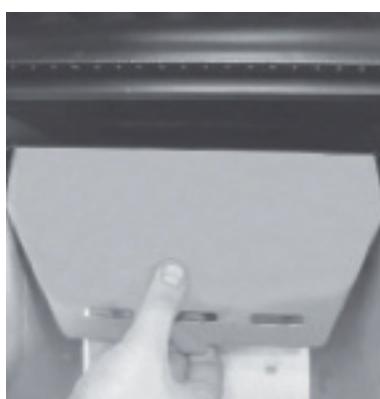
Fig. 16: rotate the fire shield
