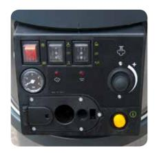
New simple and intuitive control panel, quick-coupling steam gun, main ON/OFF switch with lamp, boiler ON/OFF switch with lamp, steam function/compressed air function selector, water/detergent selector, steam flow rate regulator, steam ready indicator lamp, low water level indicator lamp with buzzer, steam pressure gauge, and air pressure gauge. Gun with integrated start-up control, adjustment of the vacuum power and
