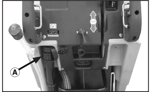
Photo 25 A) Recovery tank drain hose with adjustable drain flow
