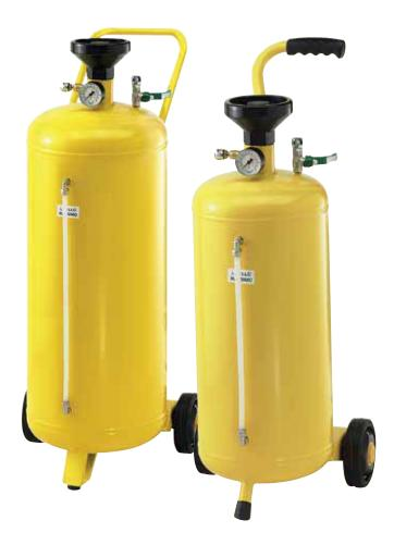
Pneumatic charge sprayers need to be connected to an air compressor to charge the tank and allow the product vaporization without the connection to the air compressor. They work at high-pressures and so they use capacious steel or stainless steel tanks to allow a greater working autonomy.
